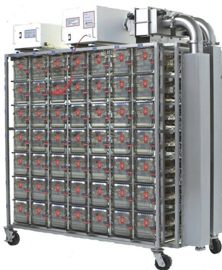
図3. IVC (Individual Ventilated Cage System)
